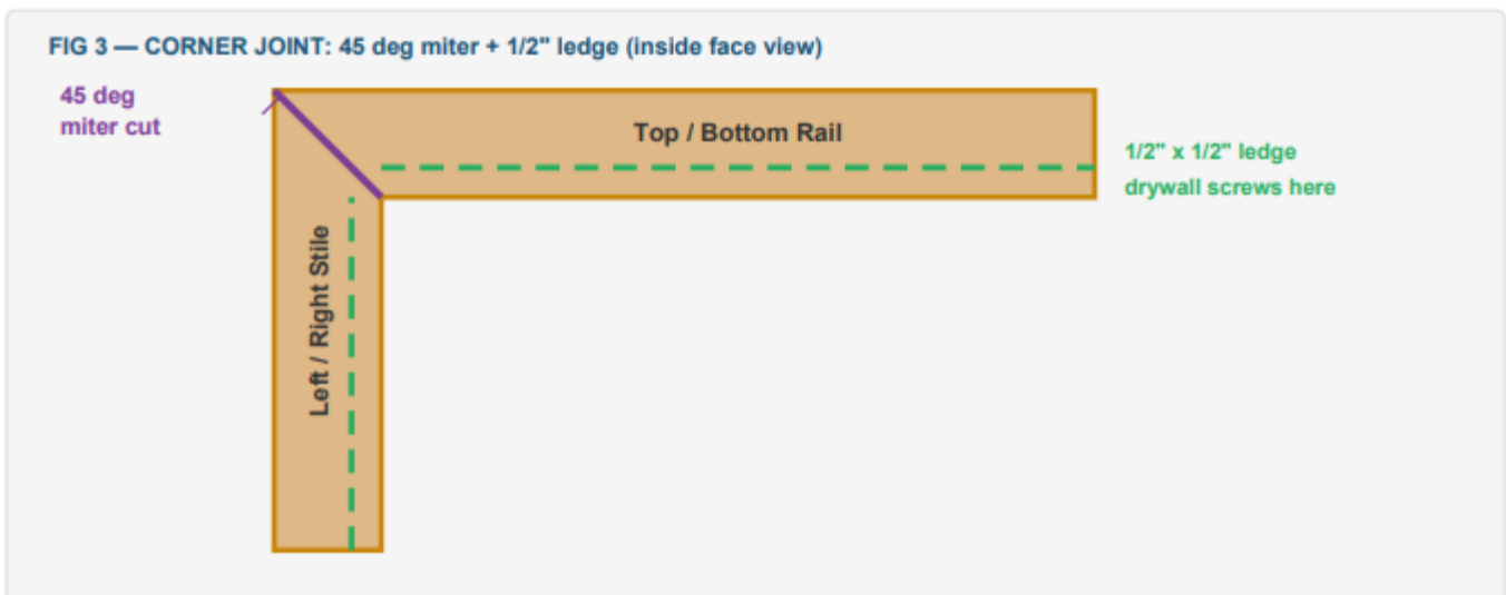
Fig 3 — Corner joint: green dashed lines = 1/2" x 1/2" interior ledge on stile and rail — drywall screws to this ledge
