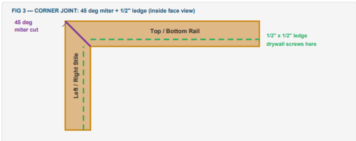
Fig 3 — Corner joint: green dashed lines = 1/2" x 1/2" interior ledge on stile and rail — drywall screws to this ledge
